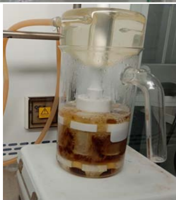
Picture: Manual filtration unit.
